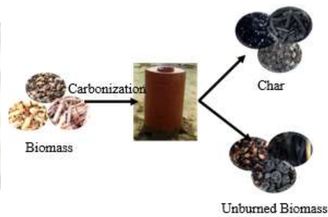
Fig. 2: Conversion of biomass into char
